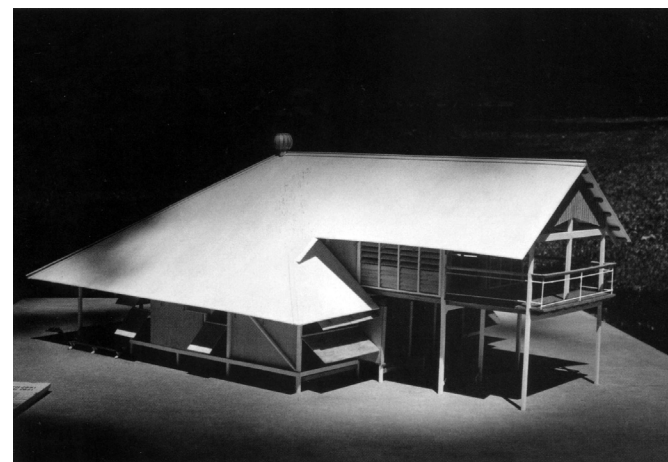
Fig. 19. Original model showing metal roof providing a large area of shade. The operable louvered wall panels can be seen, allowing occupants to have complete control over the degree to which the space is cooled by outside air. 1
